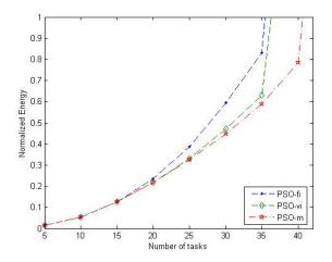
Fig. 8 A comparison among PSO-fi, PSO-vi, and PSO-m techniques with light tasks partitioned upon 4 processors.
